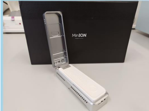
Figure 1. A single MinION flow cell generates data at a rate of 10 to 20 Gb every 48 hrs. Running multiple flow cells in parallel allows for human genome sequencing (30x coverage) in about a day.
